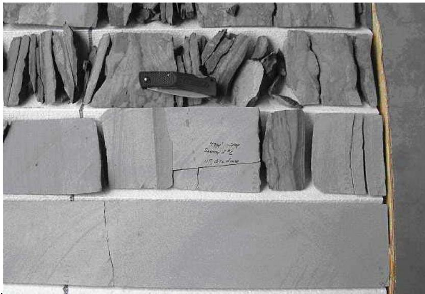
Short vertical extension fracture, terminating top and bottom at bounding lithologies.
