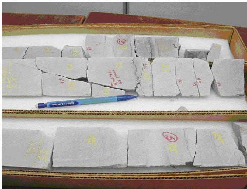
Inclined fracture (above pencil), stylolite (at pencil point) and horizontal shear planes ("HS") in the San Juan 28-238R core.
